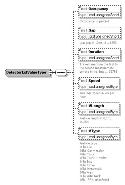
The extended detector measurements include the following elements:
